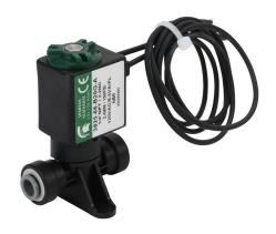
Spartan solenoid valve, 2-way, 2-position, N.C., acetal body, 1/4in push-to-connect tubing inlet(s), 1/4in push-to-connect tubing outlet(s), Cv=0.24, 150 psi maximum operating pressure, 120 VAC operating voltage, 18in 22 AWG pigtail.
