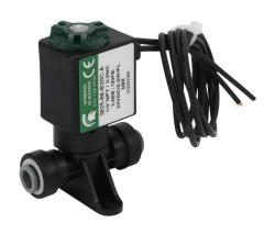
Spartan solenoid valve, 2-way, 2-position, N.C., acetal body, 1/4in push-to-connect tubing inlet(s), 1/4in push-to-connect tubing outlet(s), Cv=0.24, 150 psi maximum operating pressure, 24 VDC operating voltage, 18in 22 AWG pigtail.
