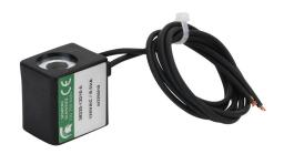
Spartan solenoid coil, 120 VAC, 8.5 VA, 18mm DIN style wiring plug. For use with 3580, 3525 and 3527 series Spartan valves.
