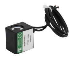
Spartan solenoid coil, 12 VDC, 6.5W, 18in 22AWG pigtail. For use with 3580, 3525 and 3527 series Spartan valves.
