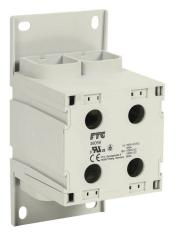
FTG enclosed terminal block, finger-safe, 840A, 1-pole, line side: 2 openings accept 600 kcmil to 4 AWG, load side: 2 openings accept 600 kcmil to 4 AWG, panel or 35mm DIN rail mount, UL 1059 recognized.
