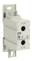
FTG enclosed terminal block, finger-safe, 355A, 1-pole, line side: 1 opening accepts 400 kcmil to 6 AWG, load side: 1 opening accepts 400 kcmil to 6 AWG, panel or 35mm DIN rail mount, UL 1059 recognized.
