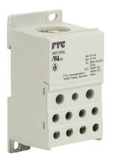
FTG enclosed terminal block, finger-safe, 310A, 1-pole, line side: 1 opening accepts 350 kcmil to 3/0 AWG, load side: 2 openings accept 2 AWG to 14 AWG & 5 openings accept 6 AWG to 14 AWG & 4 openings accept 8 AWG to 14 AWG, panel or 35mm DIN rail mount.
