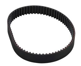
SureMotion timing belt, 5mm 5M pitch, 15mm wide, 75 tooth, 375mm pitch length (circumference), neoprene, fiberglass reinforced.
