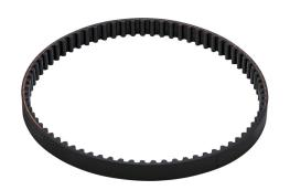
SureMotion timing belt, 5mm 5M pitch, 9mm wide, 75 tooth, 375mm pitch length (circumference), neoprene, fiberglass reinforced.
