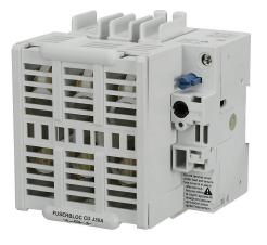
Socomec FUSERBLOC Compact series rotary disconnect switch, fusible, Class J, load break capable, 3-pole, 600 VAC, 30A, 100kA SCCR, DIN rail or panel mount, UL 489 rated, front operated, accepts 5 x 5mm size shaft, unswitched neutral.
