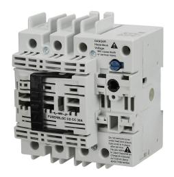
Socomec FUSERBLOC Compact series rotary disconnect switch, fusible, Class CC, load break capable, 3-pole, 600 VAC, 30A, 100kA SCCR, DIN rail or panel mount, UL 489 rated, front operated, accepts 5 x 5mm size shaft, unswitched neutral.
