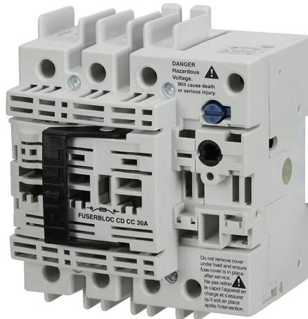
Socomec FUSERBLOC Compact series rotary disconnect switch, fusible, Class CC, load break capable, 3-pole, 600 VAC, 30A, 100kA SCCR, DIN rail or panel mount, UL 489 rated, front operated, accepts 5 x 5mm size shaft, unswitched neutral.
