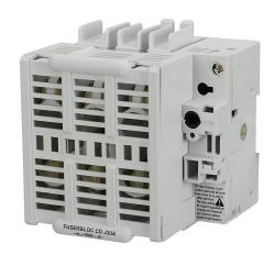
Socomec FUSERBLOC Compact series rotary disconnect switch, fusible, Class J, load break capable, 3-pole, 600 VAC, 30A, 100kA SCCR, DIN rail or panel mount, UL 489 rated, front operated, accepts 5 x 5mm size shaft, switched neutral.
