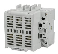
Socomec FUSERBLOC Compact series rotary disconnect switch, fusible, Class J, load break capable, 3-pole, 600 VAC, 30A, 100kA SCCR, DIN rail or panel mount, UL 489 rated, front operated, accepts 5 x 5mm size shaft, switched neutral.
