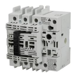
Socomec FUSERBLOC Compact series rotary disconnect switch, fusible, Class CC, load break capable, 3-pole, 600 VAC, 30A, 100kA SCCR, DIN rail or panel mount, UL 489 rated, front operated, accepts 5 x 5mm size shaft, switched neutral.
