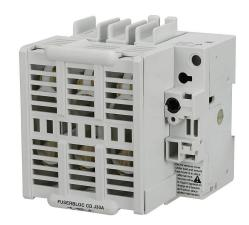
Socomec FUSERBLOC Compact series rotary disconnect switch, fusible, Class J, load break capable, 3-pole, 600 VAC, 30A, 100kA SCCR, DIN rail or panel mount, UL 489 rated, front operated, accepts 5 x 5mm size shaft.
