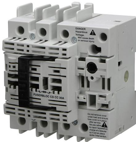
Socomec FUSERBLOC Compact series rotary disconnect switch, fusible, Class CC, load break capable, 3-pole, 600 VAC, 30A, 100kA SCCR, DIN rail or panel mount, UL 489 rated, front operated, accepts 5 x 5mm size shaft.
