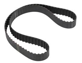
SureMotion timing belt, 3/8in L pitch, 1in wide, 98 tooth, 36.8in pitch length (circumference), neoprene, fiberglass reinforced.
