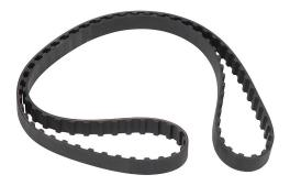
SureMotion timing belt, 3/8in L pitch, 1/2in wide, 98 tooth, 36.8in pitch length (circumference), neoprene, fiberglass reinforced.
