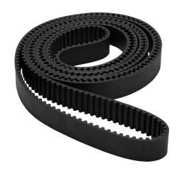
SureMotion timing belt, 8mm 8M pitch, 30mm wide, 450 tooth, 3600mm pitch length (circumference), neoprene, fiberglass reinforced.
