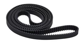
SureMotion timing belt, 8mm 8M pitch, 20mm wide, 450 tooth, 3600mm pitch length (circumference), neoprene, fiberglass reinforced.
