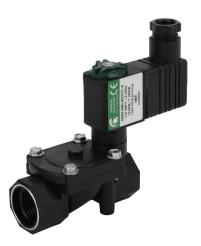
Spartan solenoid valve, 2-way, 2-position, N.C., glass-filled nylon body, 1/2in female NPT inlet(s), 1/2in female NPT outlet(s), Cv=2.45, 150 psi maximum operating pressure, 120 VAC operating voltage, 11mm DIN style wiring plug.
