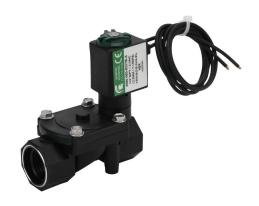
Spartan solenoid valve, 2-way, 2-position, N.C., glass-filled nylon body, 1/2in female NPT inlet(s), 1/2in female NPT outlet(s), Cv=2.45, 150 psi maximum operating pressure, 120 VAC operating voltage, 18in 22 AWG pigtail.
