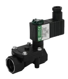
Spartan solenoid valve, 2-way, 2-position, N.C., glass-filled nylon body, 1/2in female NPT inlet(s), 1/2in female NPT outlet(s), Cv=2.45, 150 psi maximum operating pressure, 24 VDC operating voltage, 11mm DIN style wiring plug.
