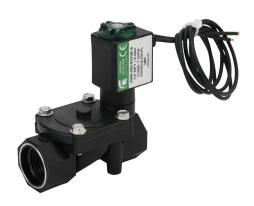
Spartan solenoid valve, 2-way, 2-position, N.C., glass-filled nylon body, 1/2in female NPT inlet(s), 1/2in female NPT outlet(s), Cv=2.45, 150 psi maximum operating pressure, 24 VDC operating voltage, 18in 22 AWG pigtail.
