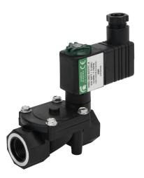
Spartan solenoid valve, 2-way, 2-position, N.C., glass-filled nylon body, 3/8in female NPT inlet(s), 3/8in female NPT outlet(s), Cv=1.95, 150 psi maximum operating pressure, 120 VAC operating voltage, 11mm DIN style wiring plug.
