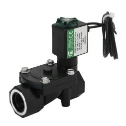
Spartan solenoid valve, 2-way, 2-position, N.C., glass-filled nylon body, 3/8in female NPT inlet(s), 3/8in female NPT outlet(s), Cv=1.95, 150 psi maximum operating pressure, 120 VAC operating voltage, 18in 22 AWG pigtail.
