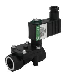
Spartan solenoid valve, 2-way, 2-position, N.C., glass-filled nylon body, 3/8in female NPT inlet(s), 3/8in female NPT outlet(s), Cv=1.95, 150 psi maximum operating pressure, 24 VDC operating voltage, 11mm DIN style wiring plug.
