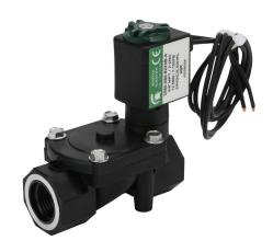
Spartan solenoid valve, 2-way, 2-position, N.C., glass-filled nylon body, 3/8in female NPT inlet(s), 3/8in female NPT outlet(s), Cv=1.95, 150 psi maximum operating pressure, 24 VDC operating voltage, 18in 22 AWG pigtail.
