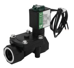
Spartan solenoid valve, 2-way, 2-position, N.C., glass-filled nylon body, 3/8in female NPT inlet(s), 3/8in female NPT outlet(s), Cv=1.95, 150 psi maximum operating pressure, 24 VDC operating voltage, 18in 22 AWG pigtail.
