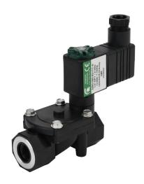
Spartan solenoid valve, 2-way, 2-position, N.C., glass-filled nylon body, 1/4in female NPT inlet(s), 1/4in female NPT outlet(s), Cv=1.55, 150 psi maximum operating pressure, 120 VAC operating voltage, 11mm DIN style wiring plug.
