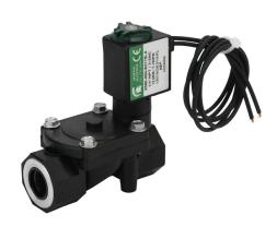
Spartan solenoid valve, 2-way, 2-position, N.C., glass-filled nylon body, 1/4in female NPT inlet(s), 1/4in female NPT outlet(s), Cv=1.55, 150 psi maximum operating pressure, 120 VAC operating voltage, 18in 22 AWG pigtail.
