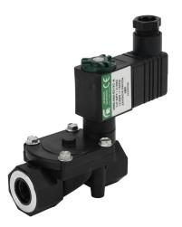
Spartan solenoid valve, 2-way, 2-position, N.C., glass-filled nylon body, 1/4in female NPT inlet(s), 1/4in female NPT outlet(s), Cv=1.55, 150 psi maximum operating pressure, 24 VDC operating voltage, 11mm DIN style wiring plug.
