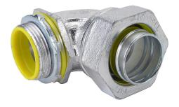
RACO connector, liquid-tight, 90-degree, 1-1/4in trade size, 1-1/4in NPT thread type, insulation, zinc electro-plated finish. Package of 10. For use with Liquatite electrical conduit. Sealing washer and locknut included.
