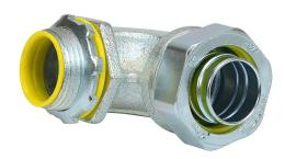
RACO connector, liquid-tight, 90-degree, 1in trade size, 1in NPT thread type, insulation, zinc electro-plated finish. Package of 10. For use with Liquatite electrical conduit. Sealing washer and locknut included.
