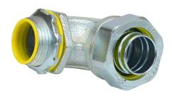
RACO connector, liquid-tight, 90-degree, 1in trade size, 1in NPT thread type, insulation, zinc electro-plated finish. For use with Liquatite electrical conduit. Sealing washer and locknut included.
