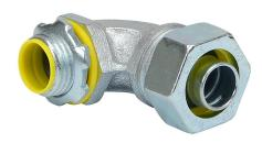
RACO connector, liquid-tight, 90-degree, 1/2in trade size, 1/2in NPT thread type, insulation, zinc electro-plated finish. For use with Liquatite electrical conduit. Sealing washer and locknut included.
