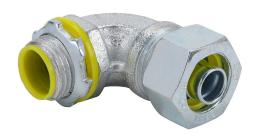
RACO connector, liquid-tight, 90-degree, 3/8in trade size, 1/2in NPT thread type, insulation, zinc electro-plated finish. Package of 25. For use with Liquatite electrical conduit. Sealing washer and locknut included.
