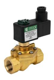
Spartan solenoid valve, 2-way, 2-position, N.C., low lead brass body, 1/2in female NPT inlet(s), 1/2in female NPT outlet(s), Cv=4.5, 180 psi maximum operating pressure, 120 VAC operating voltage, 18mm DIN style wiring plug.
