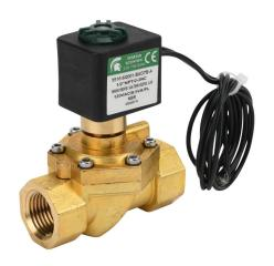
Spartan solenoid valve, 2-way, 2-position, N.C., low lead brass body, 1/2in female NPT inlet(s), 1/2in female NPT outlet(s), Cv=4.5, 180 psi maximum operating pressure, 120 VAC operating voltage, 18in 22 AWG pigtail.
