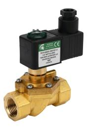
Spartan solenoid valve, 2-way, 2-position, N.C., low lead brass body, 1/2in female NPT inlet(s), 1/2in female NPT outlet(s), Cv=4.5, 180 psi maximum operating pressure, 24 VDC operating voltage, 18mm DIN style wiring plug.
