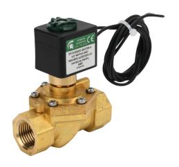
Spartan solenoid valve, 2-way, 2-position, N.C., low lead brass body, 1/2in female NPT inlet(s), 1/2in female NPT outlet(s), Cv=4.5, 180 psi maximum operating pressure, 24 VDC operating voltage, 18in 22 AWG pigtail.
