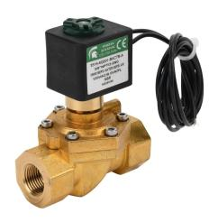
Spartan solenoid valve, 2-way, 2-position, N.C., low lead brass body, 3/8in female NPT inlet(s), 3/8in female NPT outlet(s), Cv=4.5, 180 psi maximum operating pressure, 120 VAC operating voltage, 18in 22 AWG pigtail.
