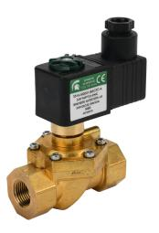
Spartan solenoid valve, 2-way, 2-position, N.C., low lead brass body, 3/8in female NPT inlet(s), 3/8in female NPT outlet(s), Cv=4.5, 180 psi maximum operating pressure, 24 VDC operating voltage, 18mm DIN style wiring plug.
