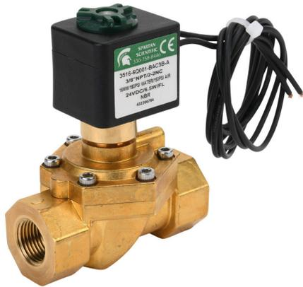
Spartan solenoid valve, 2-way, 2-position, N.C., low lead brass body, 3/8in female NPT inlet(s), 3/8in female NPT outlet(s), Cv=4.5, 180 psi maximum operating pressure, 24 VDC operating voltage, 18in 22 AWG pigtail.
