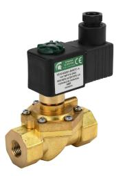
Spartan solenoid valve, 2-way, 2-position, N.C., low lead brass body, 1/4in female NPT inlet(s), 1/4in female NPT outlet(s), Cv=4.5, 180 psi maximum operating pressure, 120 VAC operating voltage, 18mm DIN style wiring plug.
