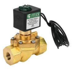
Spartan solenoid valve, 2-way, 2-position, N.C., low lead brass body, 1/4in female NPT inlet(s), 1/4in female NPT outlet(s), Cv=4.5, 180 psi maximum operating pressure, 120 VAC operating voltage, 18in 22 AWG pigtail.
