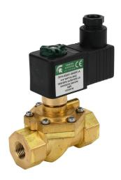
Spartan solenoid valve, 2-way, 2-position, N.C., low lead brass body, 1/4in female NPT inlet(s), 1/4in female NPT outlet(s), Cv=4.5, 180 psi maximum operating pressure, 24 VDC operating voltage, 18mm DIN style wiring plug.
