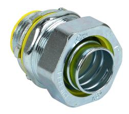
RACO connector, liquid-tight, straight, 1in trade size, 1in NPT thread type, insulation, zinc electro-plated finish. Package of 10. For use with Liquatite electrical conduit. Sealing washer and locknut included.
