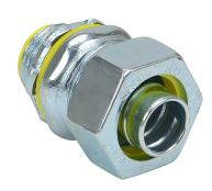
RACO connector, liquid-tight, straight, 1/2in trade size, 1/2in NPT thread type, insulation, zinc electro-plated finish. For use with Liquatite electrical conduit. Sealing washer and locknut included.
