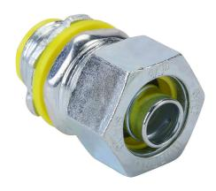
RACO connector, liquid-tight, straight, 3/8in trade size, 1/2in NPT thread type, insulation, zinc electro-plated finish. Package of 25. For use with Liquatite electrical conduit. Sealing washer and locknut included.
