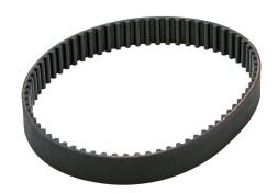
SureMotion timing belt, 5mm 5M pitch, 15mm wide, 70 tooth, 350mm pitch length (circumference), neoprene, fiberglass reinforced.
