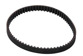
SureMotion timing belt, 5mm 5M pitch, 9mm wide, 70 tooth, 350mm pitch length (circumference), neoprene, fiberglass reinforced.
